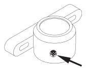
There are two different types of upper bearing housings, and each operates at a different temperature range. Verify the correct temperature range by checking the serial number on the end of the secondary shaft:
