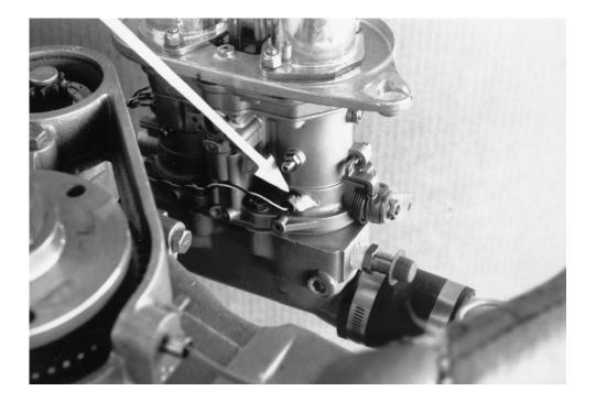
The following individual procedures are to be performed, when necessary, on the carburetor. Do not attempt to modify or change the carburetor in <u>any</u> way. The current configuration was finally determined after many hours of calibration testing on the factory dynamometer. Any jet changes necessary should be done on recommendation from a customer service representative.
