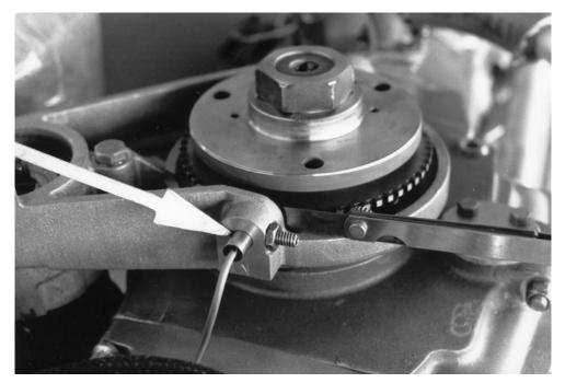
Using tie straps, secure the sender wire in such a way as to keep it from vibrating or being damaged by the heat from the exhaust. Reconnect the sender wire plug and make sure that the locking tab engages. (Route the wire according to the installation instructions.)
