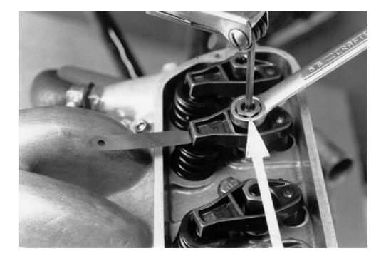
G. Rotate the engine until another valve is fully open. Measure and adjust the lash on the valve opposite it in the same manner. Continue the process until ALL of the valves are measured and adjusted.
